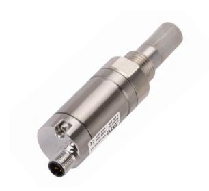
The SUTO dew point sensor S 220 provides reliable and long term stable dew point monitoring in industrial applications. SUTO is using a new sensor technology which has superior signals at very low moisture levels thus providing reliable measurements down to -100°C.
